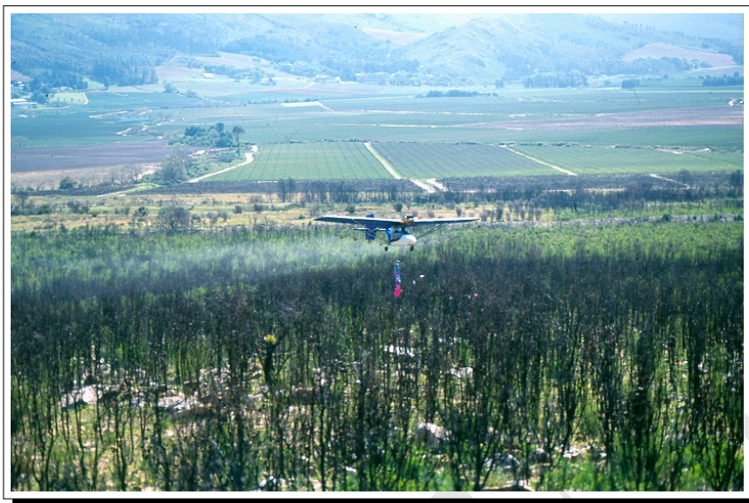
Figure 3.5: ULV-aerial application of an oil-based formulation of Colletotrichum acutatum
